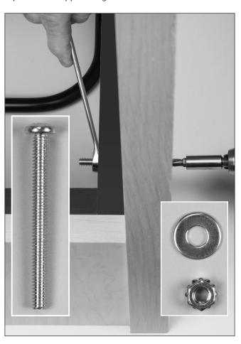
Attach the spanner by inserting the flange of the spanners into the notches in the leg.
