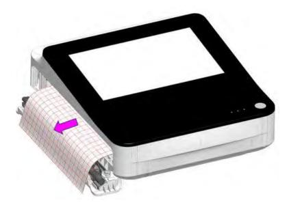
4. Push both ends of the printer door to close it and verify that the unit closes.
