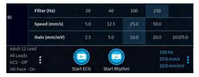
• If you purchase the **F300** - **300** Hz Acquisition option and the Acquisition Bandwidth of the selected lead set is **300Hz**, the **Filter (Hz)** value is 300.
