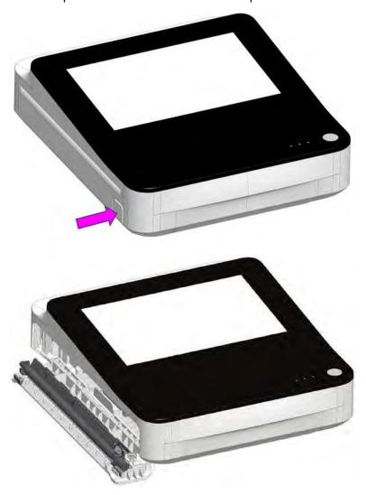
2. Pull the paper pull tab and place the paper above it, but do not remove the paper pull tab from the device. Then slide the paper into the device until it is fully inserted.
